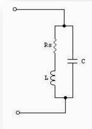
Fig.3 Equivalent circuit for a radio-frequency choke
