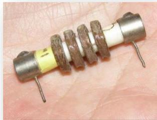
Fig.1 A four-section pi-wound 1-mH RF choke
