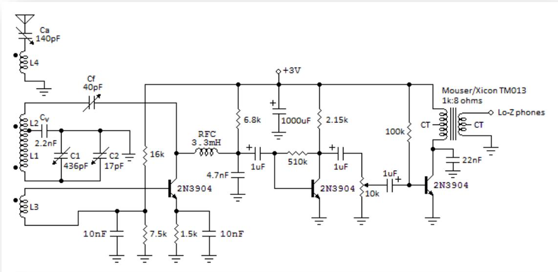
Fig.6 SW Armstrong Regenerative Receiver tunable from 3MHz to 12MHz
