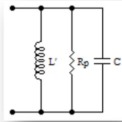
Fig.5 Equivalent circuit for an RF choke when  $Q > 5$
